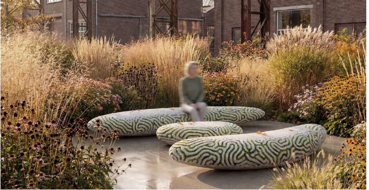
Symbio Benches (rendering), 3D printed recycled concrete
