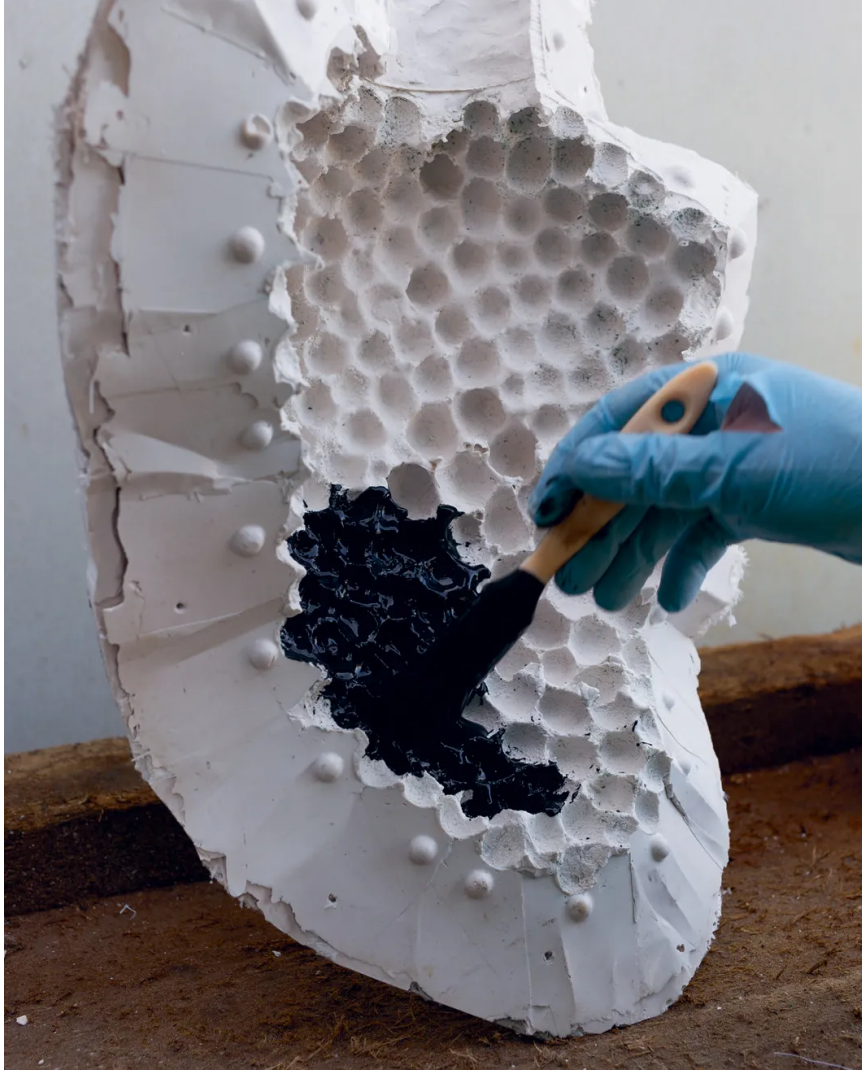
Coating the wax model in a ceramic shell (Image credit: Conor O'Leary)
