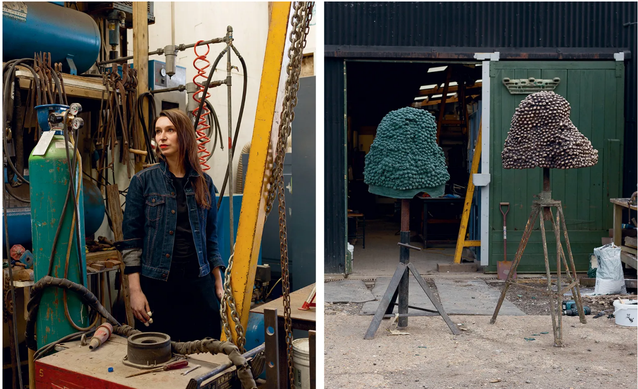
Left, Marlène Huissoud at the London Bronze Casting workshop in Farnham. Right, a wax mould before being coated in a ceramic shell, and the bronze copy of the mould. (Image credit: Conor O'Leary)
